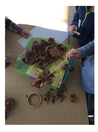
This group was not pleased with their initial results. The small slits in between the paint stirrers did cause debris to build up, making it hard for the water to flow through. The mesh helped hold the leaves, but there was nothing to move the leaves away once they had gathered. The large opening for water did work – but it worked too well! Large amounts of debris had fallen into the drain, filling it with unwanted objects.
